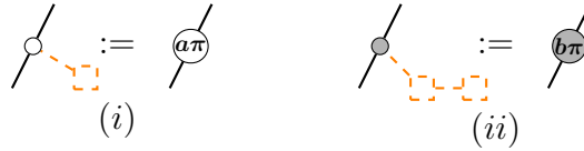
Figure 2.7: Orange dashed lines denote measurement errors. The part of diagram depicted by orange dashed line will appear if an error is produced. In (i), a Pauli Z error is depicted by a dashed orange H-box with 1 wire. In (ii), a Pauli X error is depicted by two connected dashed orange H-boxes.
